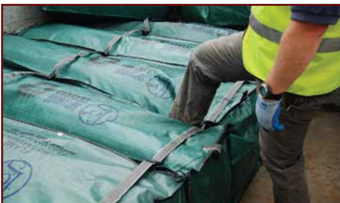
7. If the 'foot test' fails add more bags
